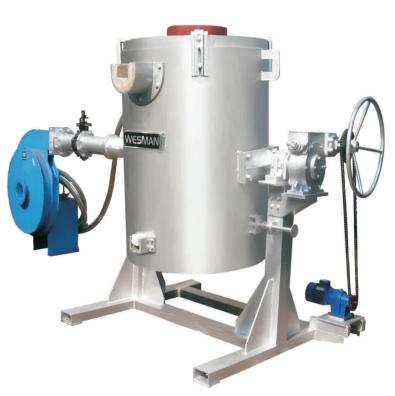
The burner fires tangentially inside the shell lining into a circular combustion space so that the hot gases surround the crucible, ensuring uniform heating. Waste gases pass out through openings at the top of the furnace, and may be collected in an optional fume extraction unit for discharge outside production area.
